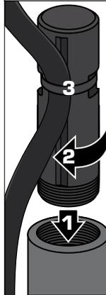
1. Screw the slug into microphone clip.
